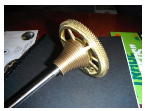
Murray Brown has been busy on his clock project and showed progress on the fusee shaft and gear wheel with spring loaded ratchet which maintains power to the gear train. He cut the gear teeth with a cycloidal cutter and the ratchet teeth with a radial saw blade. He had to fabricate a back gear train to obtain a suitable speed and torque for cutting the large gear wheel. He will be using cord on the fusee rather than chain
