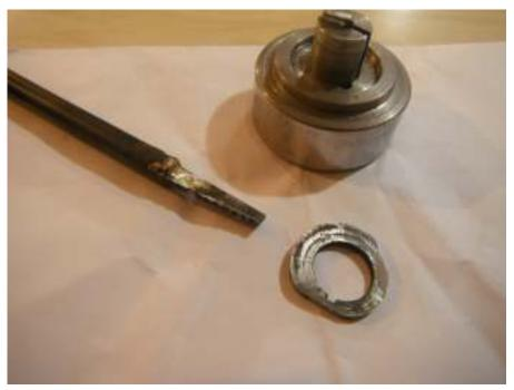
He still cant get it firing properly even after redoing the timing and suspects the valve cams may be incorrect in that the valves are not closing completely. He is in process of fabricating new cams with re-machined profiles and showed us the tool he made for broaching keyways in the new cams.
