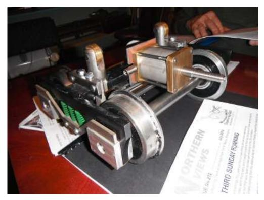
Mark Taylor has been working on a number of projects including his Phantom tender bogey on which he has fitted an air brake cylinder and actuating levers/cam mechanism. The valve block on the converted steam pump has been causing problems and he has outsourced the production of this. He has been working
